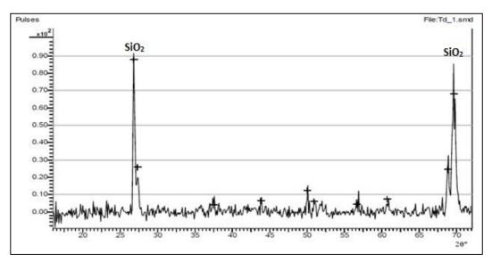
Plate 4: XRD spectrum for Quartz
