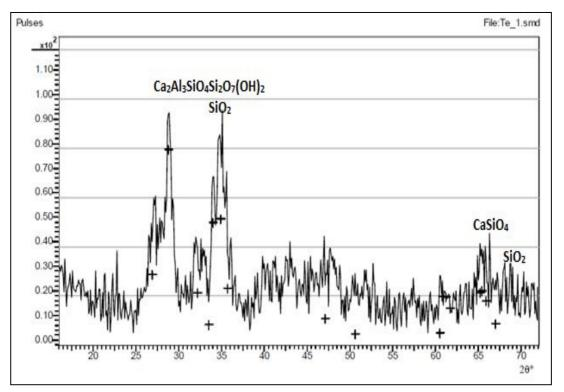
Plate 5: XRD spectrum for Wood ash
