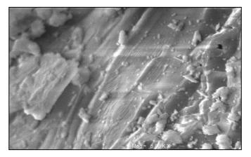
Plate 9: SEM of porcelainised stoneware tile with (kaolinitic clay) 5% wood ash M X 5000
