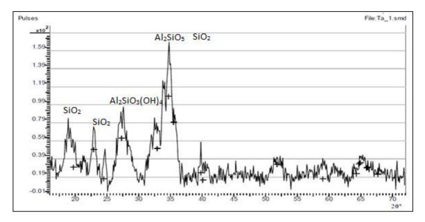
Plate 1: XRD spectrum for Kaolinitic clay.
