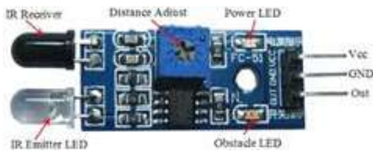
Figure 3: IR Proximity Sensor
