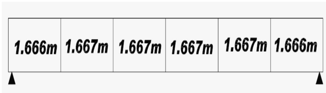
Figure (1b): A discretized uniform beam
